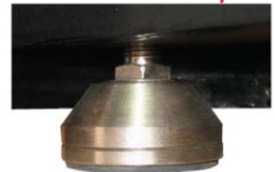
Stainless steel feet with rubber bottoms are attached to each load cell – ball-in-cup design makes feet self-swiveling and base easier to install
